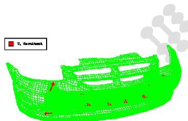
Reduced surface adjustments with shell contact thickness reduced
