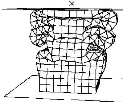
Final deformed mesh shows smooth folds, as expected.
