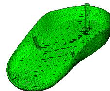
Mouse casing meshed with C3D10M elements
